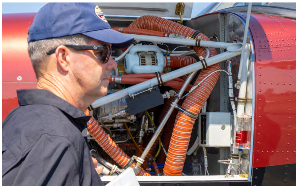
Daher selected the PT6-140A, which easily produces 900 HP. That's 200 more horsepower (in cruise) than the Kodiak 100.
