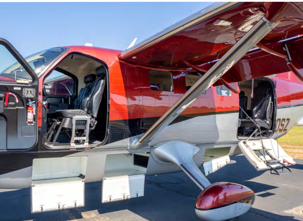
The Kodiak 900 measures 4.5 feet longer than the Kodiak 100 and incorporates several aerodynamic improvements, such as wheel fairings.
