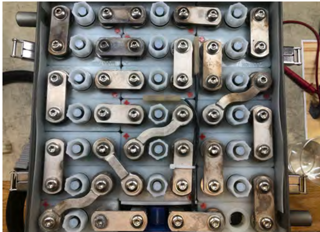
A NiCad battery with Cadmium plated hardware isn't immune to the effects of corrosion.
