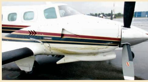
What started as a deferred maintenance issue – a small oil leak – on Kevin Dingman's Beechcraft Duke led to a drop in oil pressure. This required an inflight engine shutdown and landing to LPV minimums in rain.
