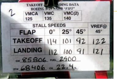
FiFi's TOLD card for a lightly loaded short flight at 86,000 pounds, nearly 25,000 pounds below gross weight. She was loaded at just over half tanks, with 2,900 gallons of 100LL on board.
