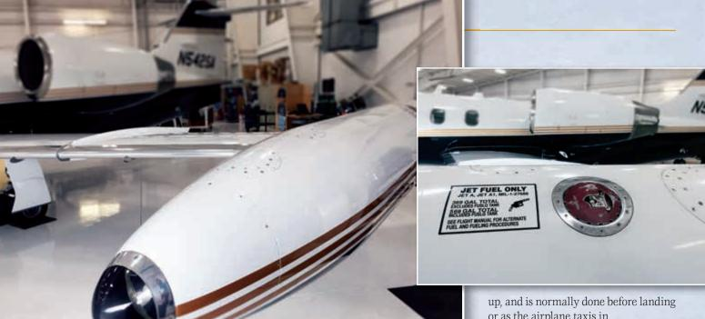
The Learjet 35 contains its fuel in two tip tanks, two wing tanks and an aft fuselage tank. The fueling process requires special care that one tip tank is not filled while the other remains empty.
