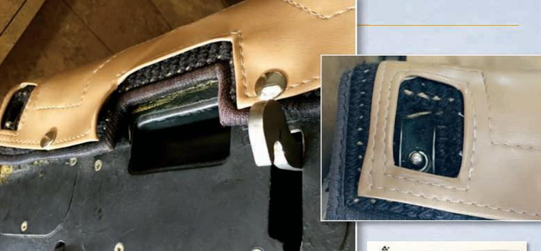
The partially-hidden toggle switch (pictured at right) operates an electrically operated hook that latches the clamshell door together (above). Not following proper door-closing procedure will lead to a potentially dangerous "gotcha."
