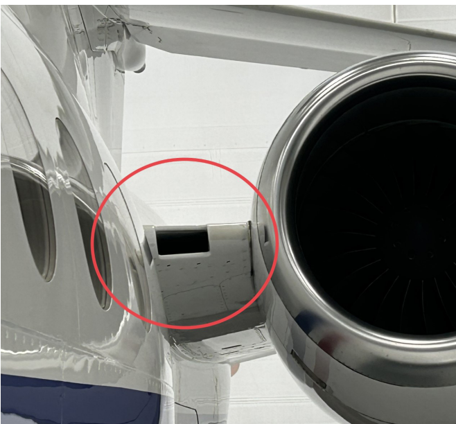
A ram air scoop feeds the ACM on this Falcon 900LX
