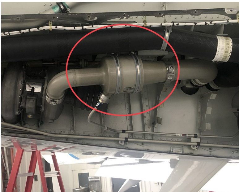
A water separator “demoisturizes by centrifuging.”
