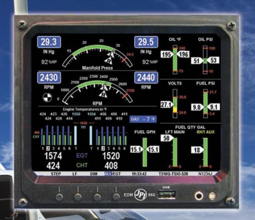
The EDM960 is certified as a primary flight instrument. The 960 can open up space in your panel, allow precise engine management, and log performance history. Spot engine trends before they become problems. JPI's EDM 960 is always monitoring your twin's engine performance.
