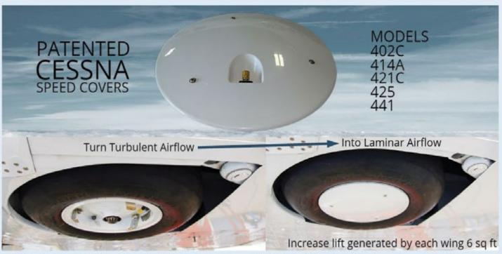
Most Cost-Effective STC to Increase Safety, Climb, Cruise Speed, Range, and Fuel Economy for Hydraulic Gear Twin Cessnas
