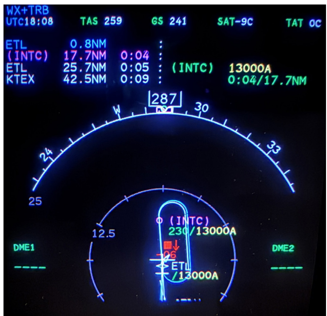
Fig 7. Pro Line 4 TCAS RA on MFD
