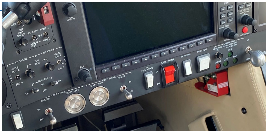
The business end of a DA62. ECU voter and alternator switches on the left
