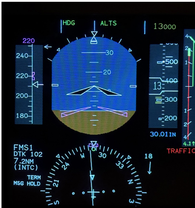
Fig 5. Pro Line 4 TCAS RA on PFD
