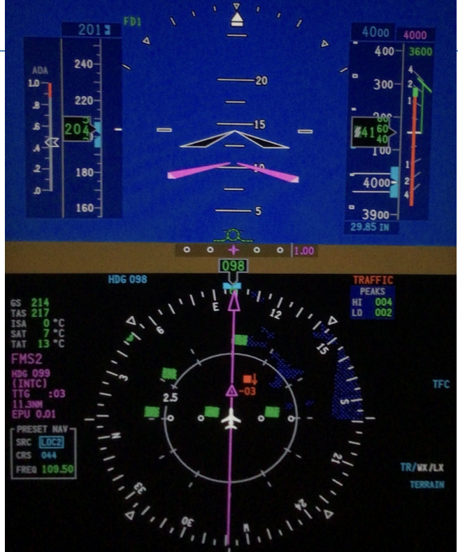
Fig 6. Pro Line 21 TCAS RA on PFD
