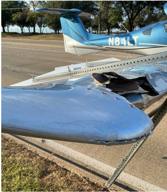
The landing was a success, but the wing was heavily damaged by a road sign
