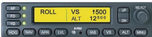
The S-TEC 3100 digital, attitude-based autopilot is one of the most advanced autopilots ever developed for general aviation. You can now be confident of precise digital control for every phase of flight, with features such as envelope protection\*, straight and level recovery, altitude preselect\*, precision approaches and much more. The S-TEC 3100 interfaces with compatible EFIS displays and analog gauges.
