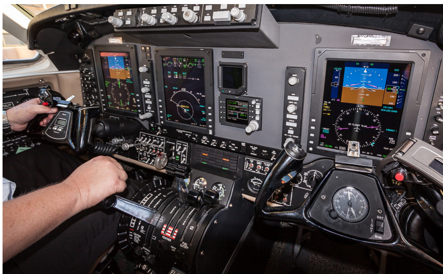
The typical King Air panel configuration with autopilot controls at the top.
