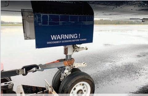
The G150 nose wheel steering system has a pin that is pulled when parked and must be re-inserted before taxi, a task that is sometimes easier said than done.
