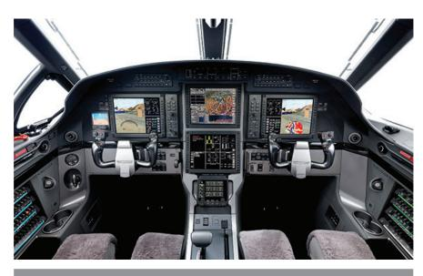
With the new servo-controlled PCL, the pilot can set a speed and the system maintains it. It is another feature that reduces workload – especially when ATC requests a specific speed, or you are flying a speed-restricted departure or arrival procedure.
