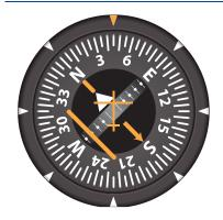
Figure 1: Landing on Runway 18, I have the HSI course needle pointing on runway heading. My downwind course will be in the opposite direction, 360. My current heading of about 045 degrees is correct for a 45-degree entry to the downwind.
