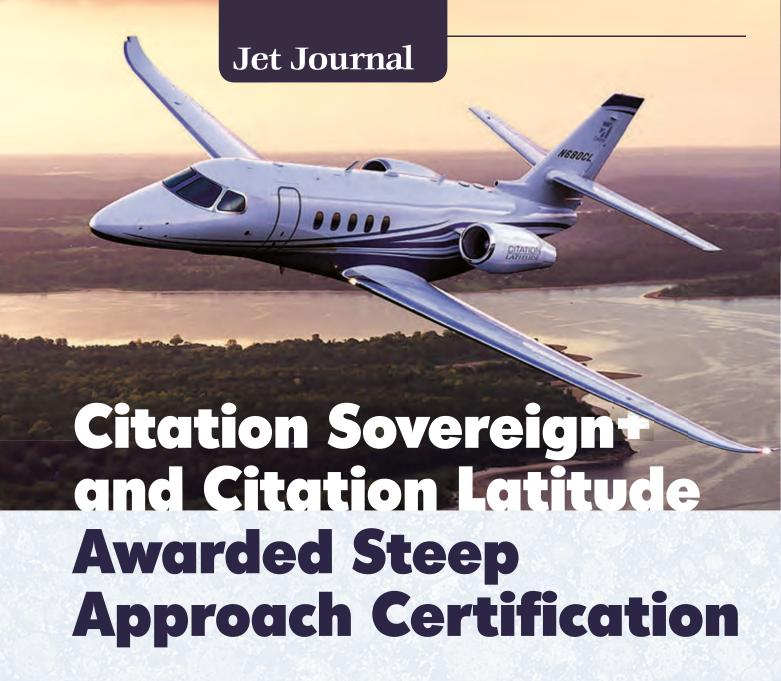
he Cessna Citation Sovereign+ and the Citation Latitude have attained FAA and EASA steep approach certification, adding operational capability to the midsize business jets. The certification allows the aircraft to fly approach angles of up to 6.65 degrees, which is necessary to access European destinations such as London City Airport (LCY) and Lugano Airport (LUG) in Switzerland. The steep approach capability for both Cessna Citation models will come standard.
